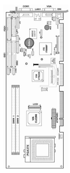
PSB-1688LF Connector, Jumper and Component locations
